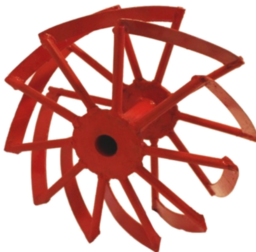
Figure 7 – Rotary working element with elliptical cutting blades
