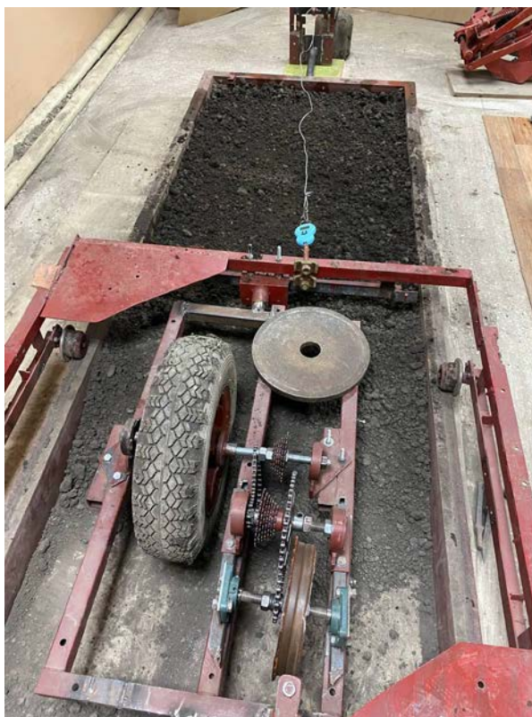
Figure 4 – Laboratory test rig with actively-driven wheel
