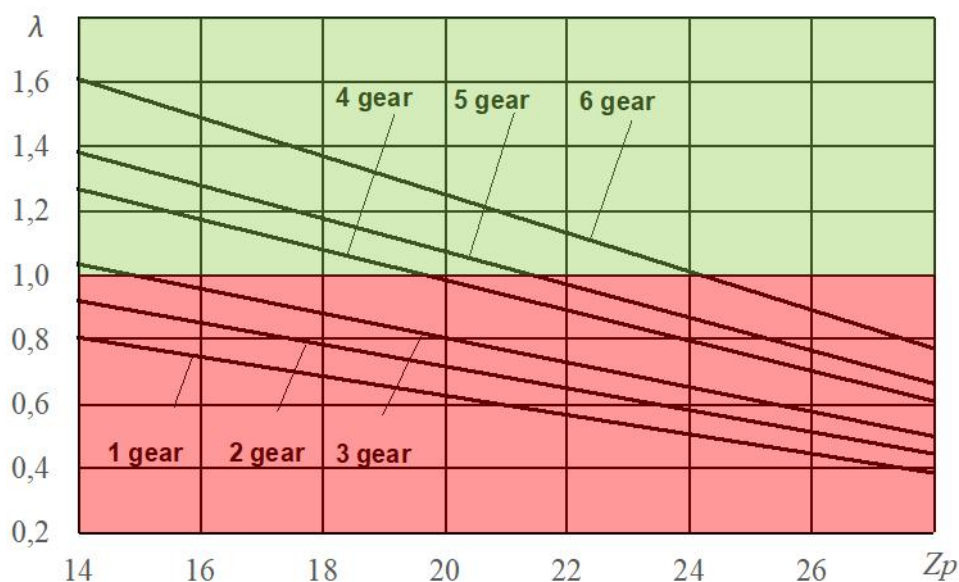
Figure 5 – Dependencies of the coefficient of kinematic mode of wheel rotation \lambda on the number of teeth of the interchangeable drive sprockets Z_6/Z_p
