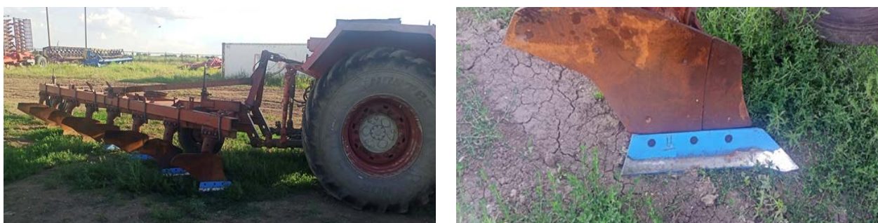
Figure 7 – Mounted plow PLN-8-35 and general view of the installed share
