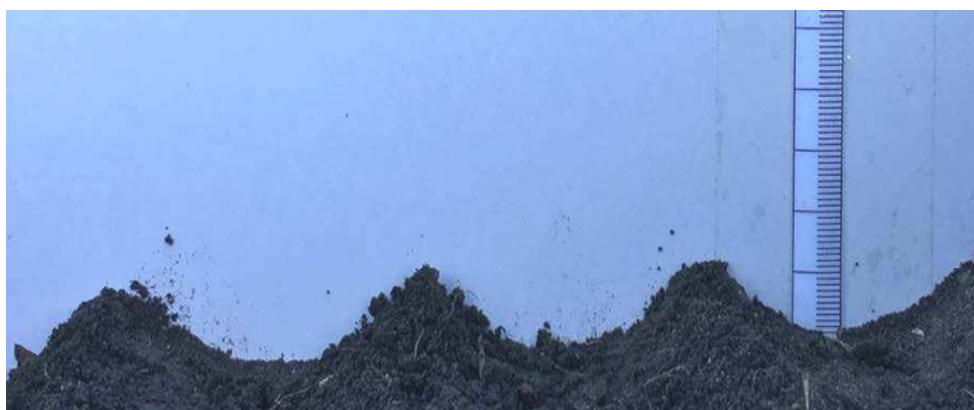
Figure 6 – Profile of the furrow bottom after the passage of the implement
